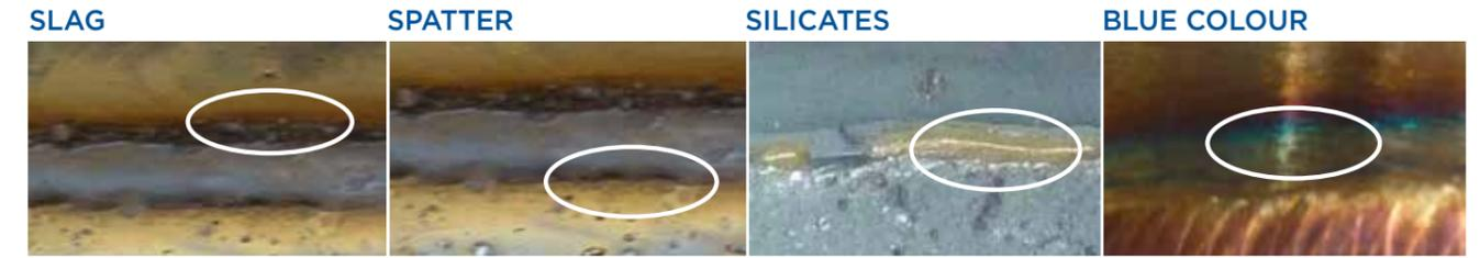
Most common contaminations occurring in a welding process.
